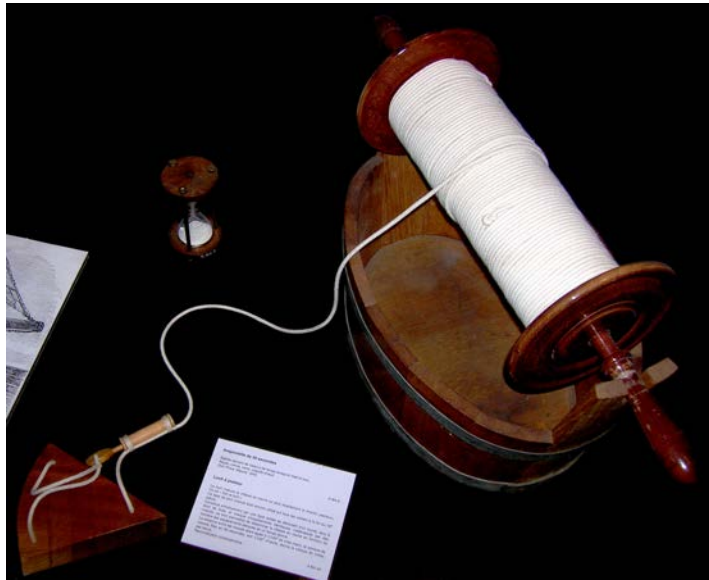
Figure 2.1: A “chip log”, used for shipborne speed estimation. ©Rémi Kaupp [23]
