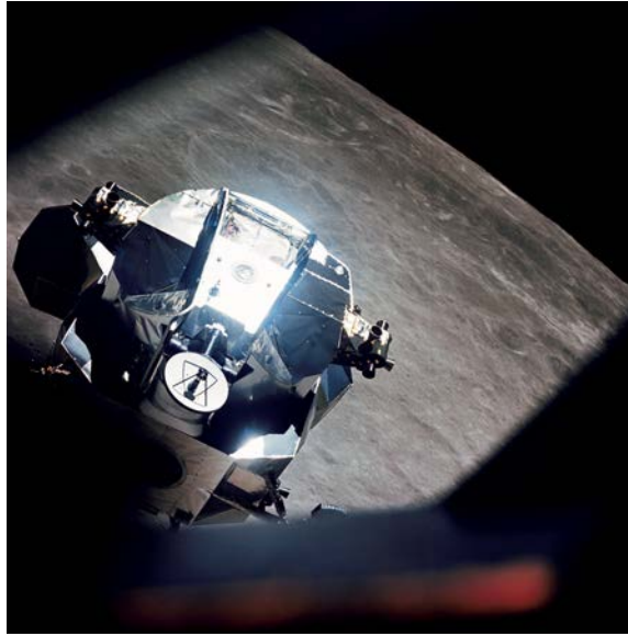
Figure 4.1: Apollo 10 Lunar Module Snoopy as seen from Command Module Charlie Brown shortly before rendezvous in lunar orbit. A Kalman filter onboard Snoopy converted radar and IMU measurements into the precise relative navigation solution required for a successful rendezvous [13]. Public-domain image courtesy of NASA [77].
